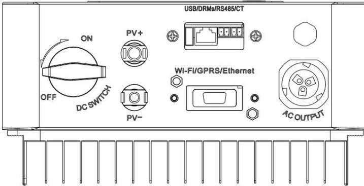
Table 4-3 Recommended communication cable size are shown below, The wiring methods are the same for RS485 and CT, this part describes their wiring methods and logic interface wiring method.
