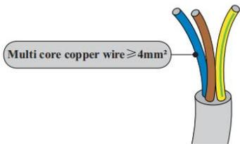
AC cable should be correctly sized to ensure the power loss in AC cable is less than 1% of the rated power. If the resistance of the AC cable is too high, it will cause a huge increase in the AC voltage, which may lead to a disconnection of the inverter from the electrical grid. The
