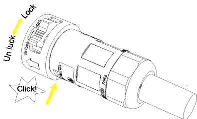
**Step 5** Connect the connected AC connector to the AC connector of the inverter. Turn the ac connector knob to lock until you hear a "click" and the clasp is in place.
