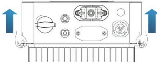
**Step 2** Lift the SOFAR 1.1K~3.3KTL-G3 from the packing case and move it to the
