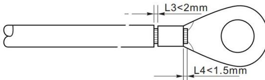
**Note 1:** L3 is the length between the insulation layer of the ground cable and the crimped part. L4 is the distance between the crimped part and core wires protruding from the crimped part.
