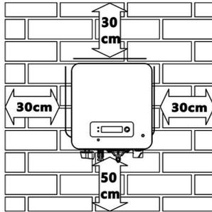
Figure 3-5 Installation of multiple SOFAR 1.1K~3.3KTL-G3 inverter
