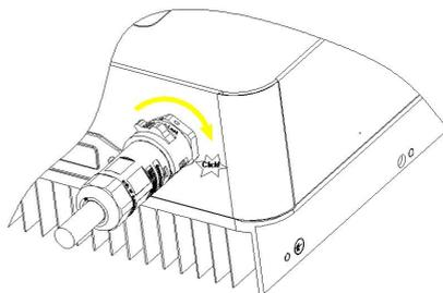
**Removing the AC connector** Hold the button to unlock and rotate the knob counterclockwise to the unlock position, then pull out the AC connector.
