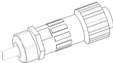
**Step 5** Connect the AC connector to the output wiring connector of inverter, rotate the AC connector clockwise until the fastener reaches its designated position, as shown below.
