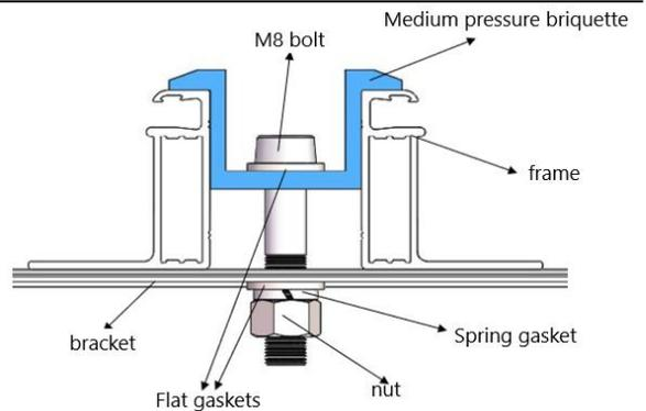
Fig. 10 Installation schematic diagram of mid clamp
