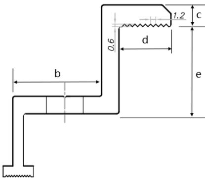
Fig. 8 Cross section diagram of fringe clamp
