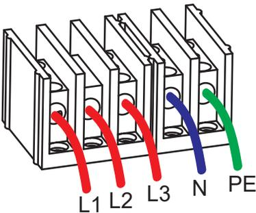
Pic 5.9 AC cable connected to the terminal
