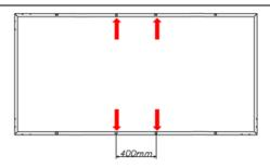
Fig. 8 66cell PV module 400mm spacing bolt installation
