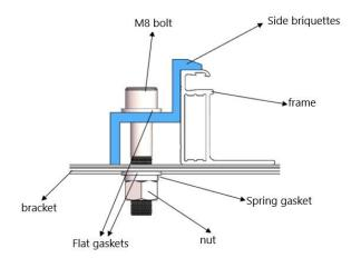
Figure 16 Installation schematic diagram of fringe clamp
