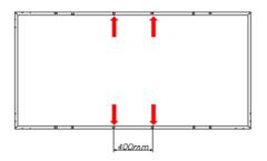
Fig. 9 72cell PV module 400mm spacing bolt installation
