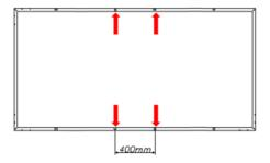
Fig. 7 60cell PV module 400mm spacing bolt installation
