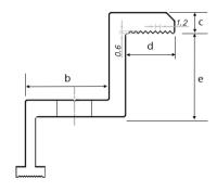
Figure 15 Cross section diagram of fringe clamp
