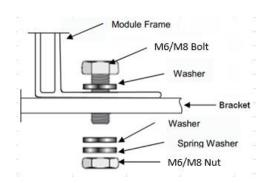
Fig. 10 Diagram of the bolt installation process
