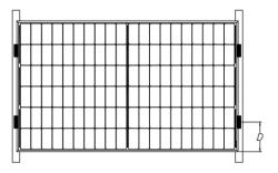
Fig. 12 Rails overlapping the short-side frame
