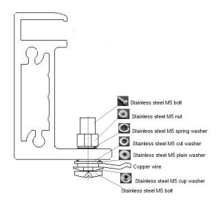
Fig. 19 Grounding the aluminum frame with copper wire
