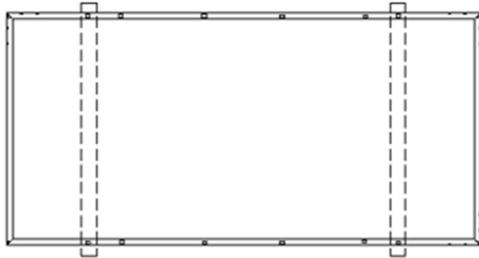
Fig. 5 Outer four-hole bolt installation for 72cell
