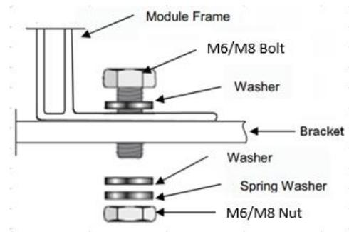
Fig. 10 Diagram of the bolt installation process
