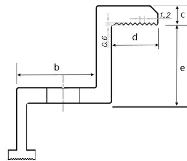
Figure 15 Cross section diagram of fringe clamp
