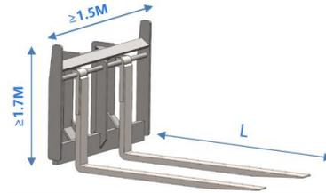
Backrest: height  $\geq 1.7m$ , width  $\geq 1.5m$
