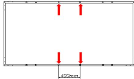
Fig. 9 72cell PV module 400mm spacing bolt installation
