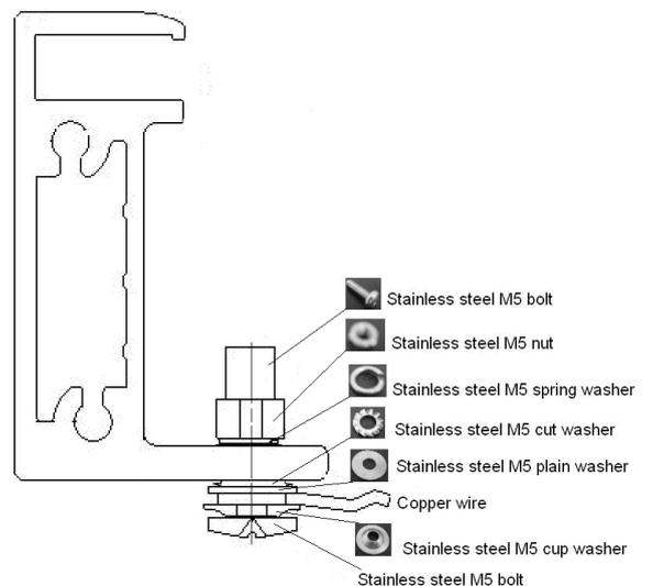
Fig. 19 Grounding the aluminum frame with copper wire
