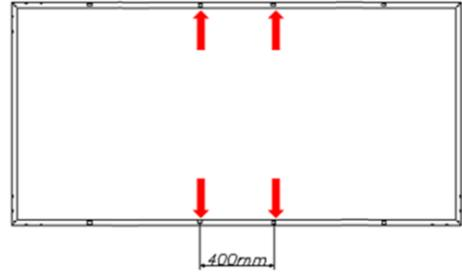
Fig. 8 66cell PV module 400mm spacing bolt installation
