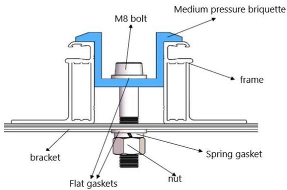
Figure 17 Installation schematic diagram of mid clamp
